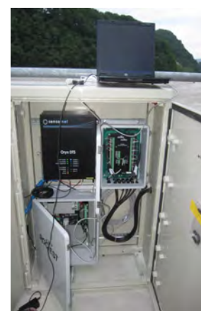
Heating modules on the left and reading units and modem on the right
