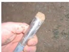
Piezometer with soil on the tip and hybrid cable
